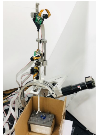
Fig. 2. LapaRobot [7] installed with a forcep for executing teleoperated surgical tasks.
