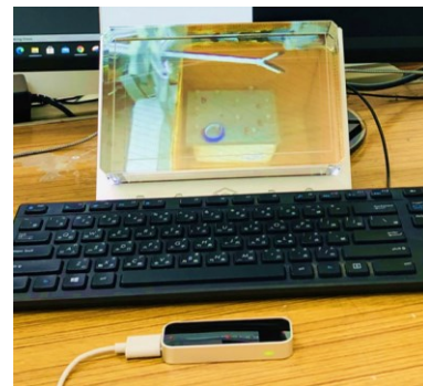
Fig. 3. Advanced remote control interface consists of a 3D hologram display (Looking Glass 8.9", Looking Glass Factory, Brooklyn, NY) and a hand gesture tracker (Leap Motion Controller, Ultraleap, Mountain View, CA).
